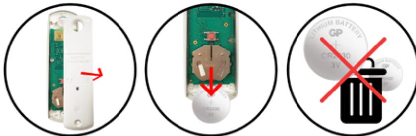
1. Using a small screwdriver loosen the screws on the reverse side of the remote control and remove the back cover.
