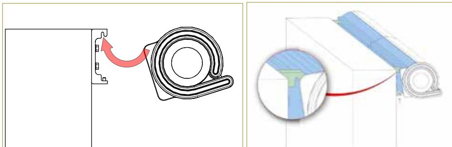
Finally, fix the product by M6x12mm stay bolt to wall bracket.
