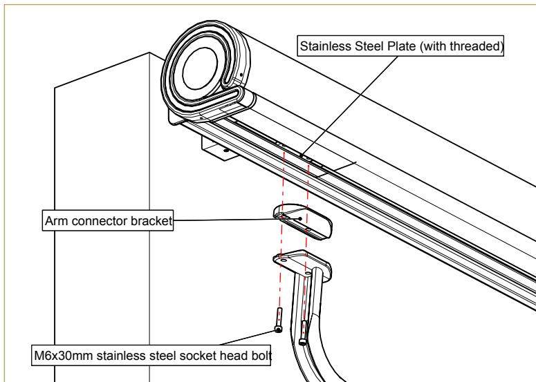
The arms should be behind of the terminal profile. Fix the arms by M6x30mm socket head bolt to steel plate inside of the terminal profile.
