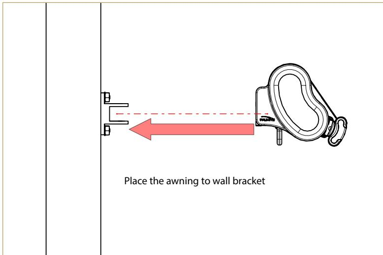
Finally, fix the product by M8x60mm hexagonal head bolt to wall bracket.
